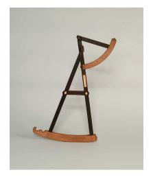
EARLY DAVIS STYLE BACKSTAFF "MADE FOR MR. JOSEPH LIGHT". Backstaff is made of various woods including mahogany and holly. Inset ivory plaque and diamonds. Carved scales. SIZE: 20.25in CONDITION: Missing slide to each scale, point at which top scale meets staff has broken and parts missing, in need of repair
